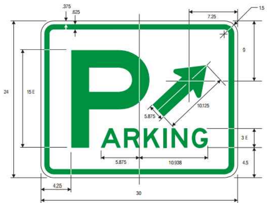
D4-1 PARKING AREA
